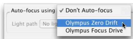
N.B. The “Using light path” field may be set to “None”, however, if you want to ensure that the specimen is not illuminated during auto-focussing you should select a light path that closes the appropriate shutter.
